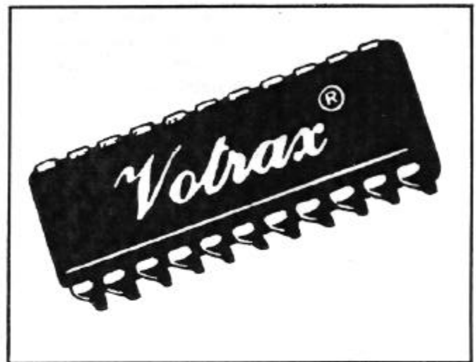
Figure 1. Votrax® SC-01 Speech Synthesizer
